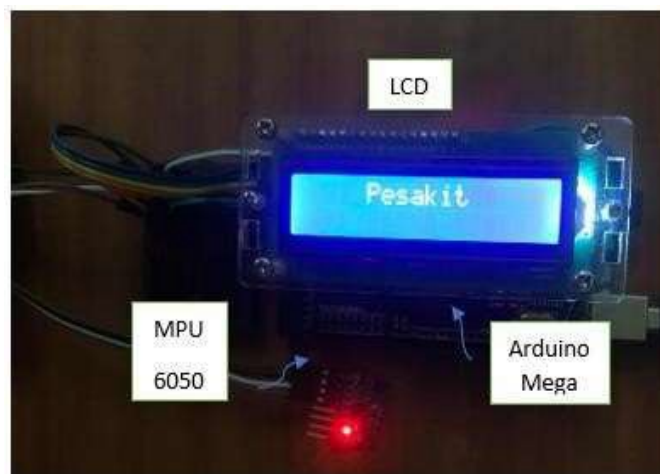
Fig. 9 - Message conveyer hardware circuit for people with disabilities
