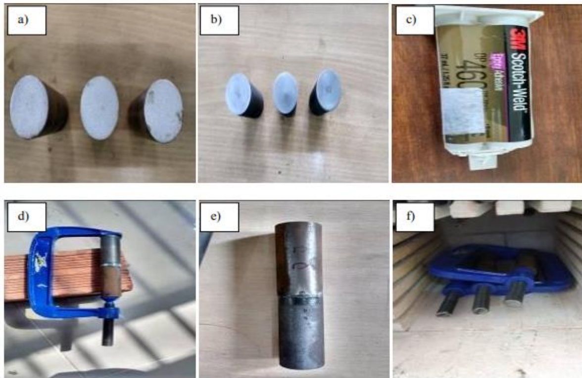
Fig.3. Specimen prepared for adhesion strength a) with coating b) without coating c) adhesive glue d) holding the specimen in C-clamp e) specimen joined for test f) specimen kept at the furnace for curing.
