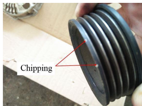
Fig. 5 - Chipping on pulley
