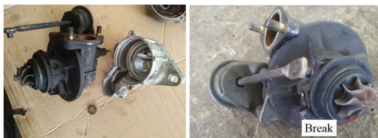
Fig. 4 - Turbocharger and its typical damaged parts
