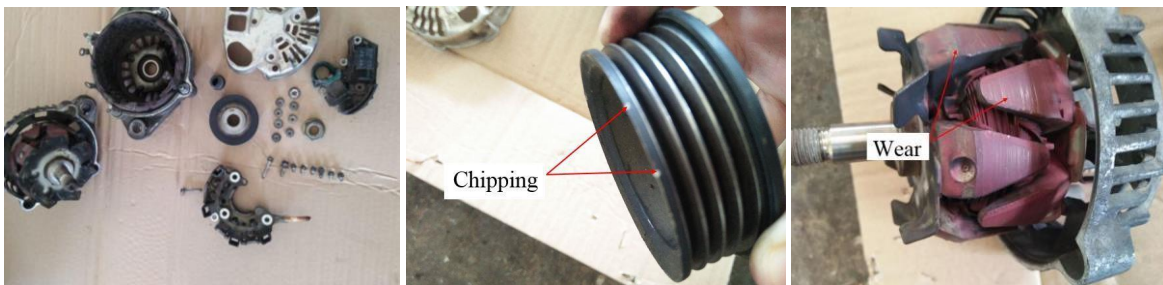
Fig. 2 - Alternator and its typical damaged parts
