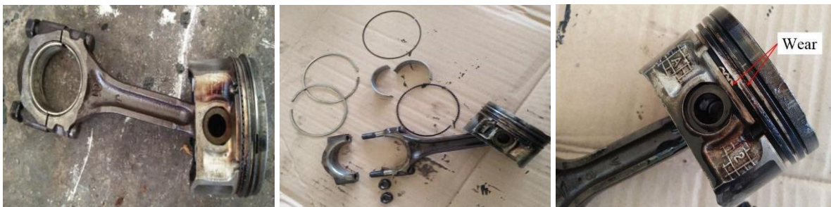
Fig. 3 - Piston and its typical damaged parts
