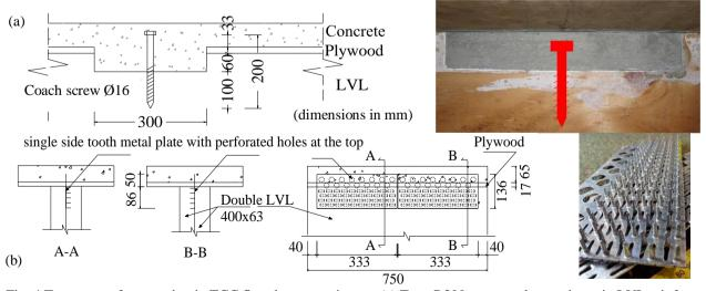
Fig. 4 Two types of connection in TCC floor beam specimens: (a) Type R300, rectangular notch cut in LVL reinforced with Ø16 mm coach screw; (b) Type P, toothed metal plates pressed into the lateral face of the LVL
