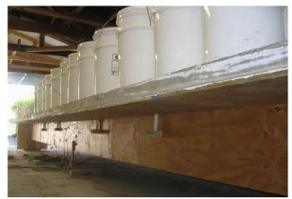
Fig. 5 TCC floor beams under long-term quasipermanent using water buckets.
