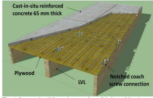
Fig. 1 Innovative M-section semi-prefabricated laminated veneer lumber (LVL)-concrete composite floor system developed in University of Canterbury.
