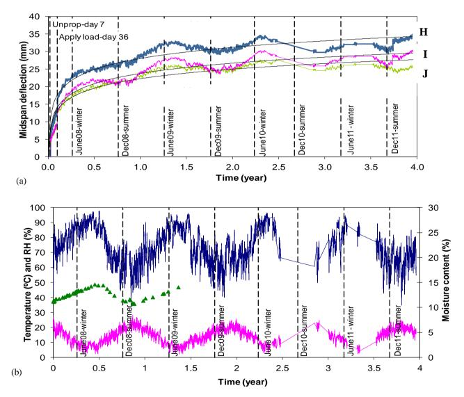
Fig. 7 (a) Mid-span deflection of beams H, I and J under long-term load from 25<sup>th</sup> February 2008 to 13<sup>th</sup> March 2012 and analytical fitted curves using logarithmic function equations, and (b) Relative humidity, temperature, and average LVL moisture content changes throughout the long-term tests.
