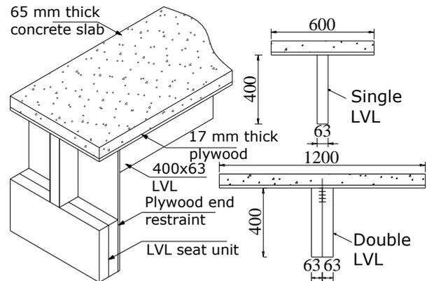
Fig. 3 LVL seats to simply support the TCC floor beam specimens and, the width for single and double LVL TCC floor beams.
