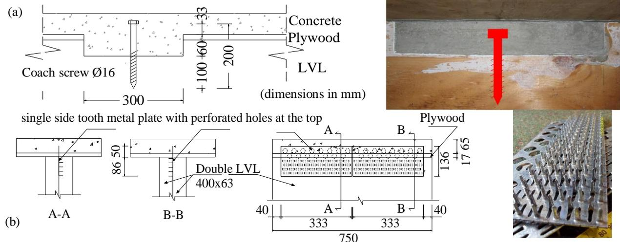
Fig. 4 Two types of connection in TCC floor beam specimens: (a) Type R300, rectangular notch cut in LVL reinforced with  $\varnothing 16$  mm coach screw; (b) Type P, toothed metal plates pressed into the lateral face of the LVL
