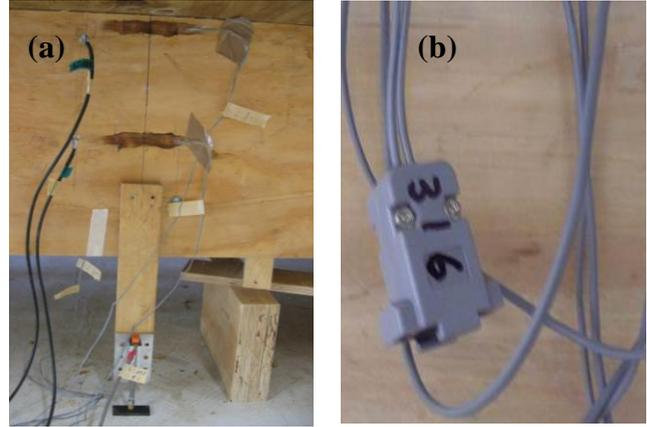
Fig. 6 Instrumentation on specimens (a) Potentiometer and strain gauges at mid span to measure displacement and strain, respectively; (b) Sensors for humidity (HIH4000) and temperature (LM35CA).
