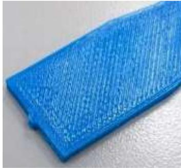
**Fig. 14 - Modification specimen at nozzle Z level point by semicircle at grips contact zones**
