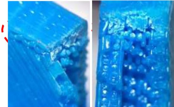
**Fig. 11 - Spacesleft near the edge at the printed specimen**
