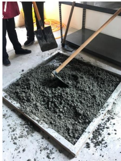
Fig. 3 - Fresh EPS-POFA concrete
