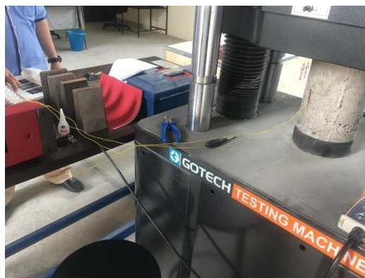
Fig. 5 - Test set-up for stress-strain curve testing
