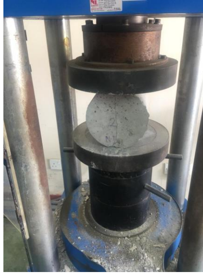
Fig. 4 - Splitting tensile strength test setup
