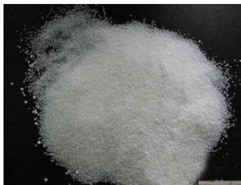
Fig. 2- Expanded polystyrene (EPS)
