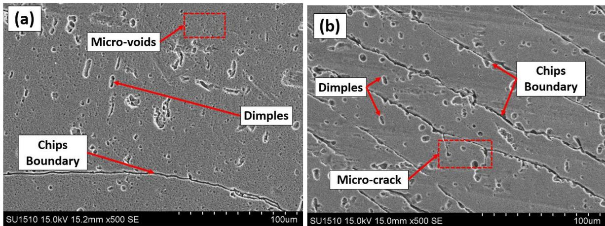
**Fig. 7 - SEM micrographs of recycled AA6061 (a) before and (b) after (100 °C,  $5.8 \times 10^{-4} \text{ s}^{-1}$ )**
