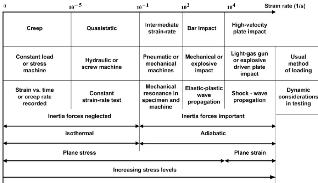
Fig. 1 - Classification of mechanical dynamic testing
