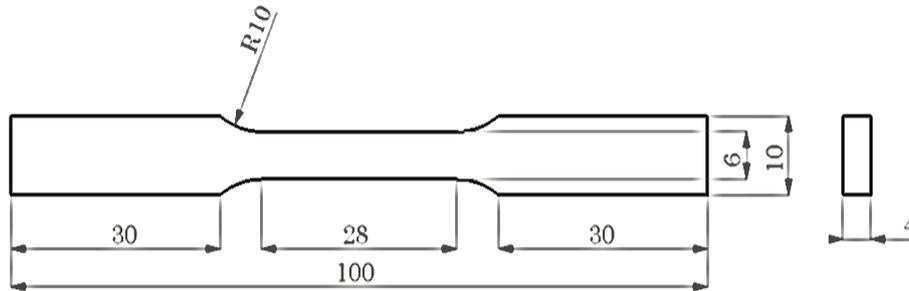
**Fig. 3 - Standard geometric of ASTM E21**
