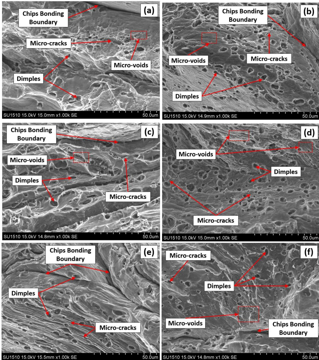
**Fig. 8 - SEM micrographs of fracture surface of specimen tested at: (a) 100 °C &  $5.8 \times 10^{-4}$  /s; (b) 100 °C &  $5.8 \times 10^{-3}$  /s; (c) 200 °C &  $5.8 \times 10^{-4}$  /s; (d) 200 °C &  $5.8 \times 10^{-3}$  /s; (e) 300 °C &  $5.8 \times 10^{-4}$  /s; (f) 300 °C &  $5.8 \times 10^{-3}$  /s**
