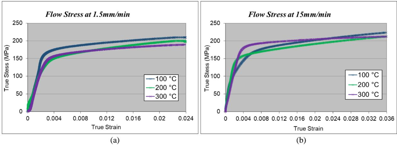
**Fig. 6 - Stress-strain curves of recycled AA6061-T5 at various temperature at loading speed of: (a) 1.5 mm/min; (b) 15 mm/min**
