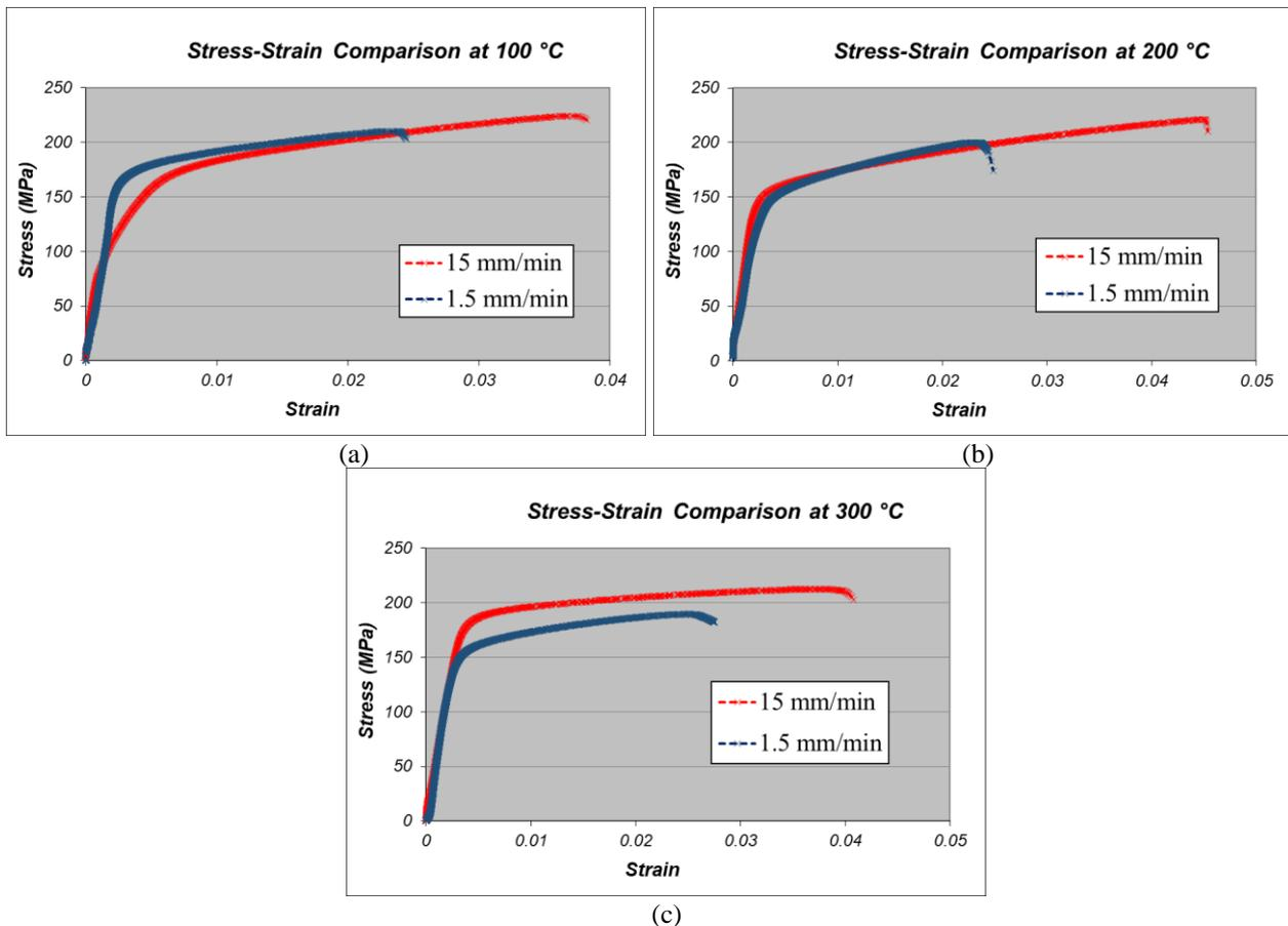
Fig. 5 – Stress-strain curves of recycled AA6061-T5 at different temperature: (a) 100 °C; (b) 200°C; (c) 300 °C
