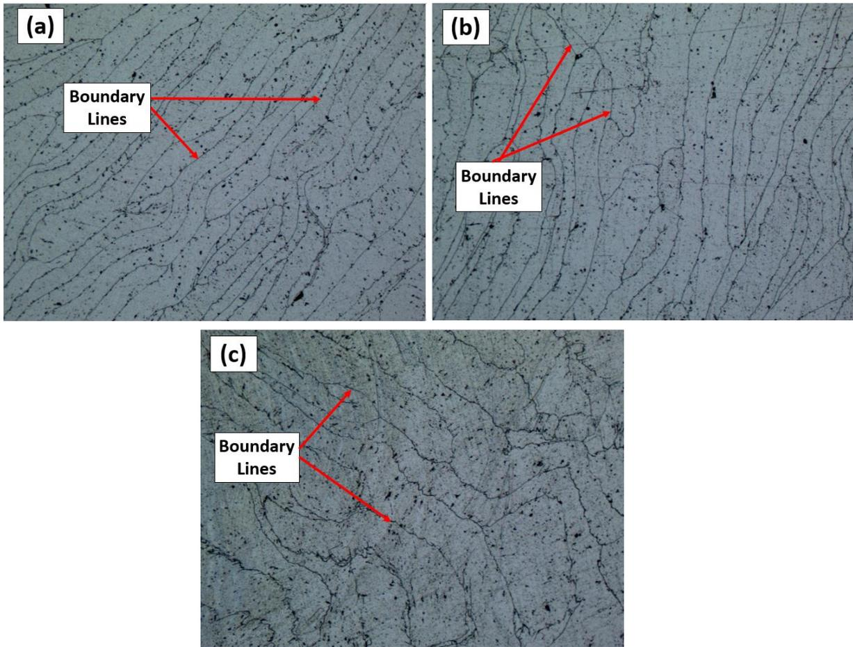
**Fig. 9 - OM micrographs of recycled AA6061 at strain rate of  $5.8 \times 10^{-4}$  at temperature of: (a) 100 °C; (b) 200 °C; (c) 300 °C**
