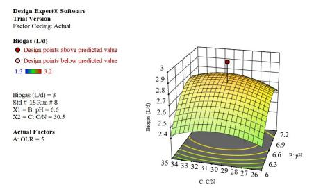
Fig. 5 - Biogas production optimization with respect to pH and C/N
