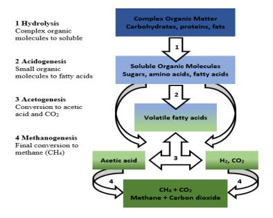
Fig. 1 - Biogas production from POME [7], [24]
