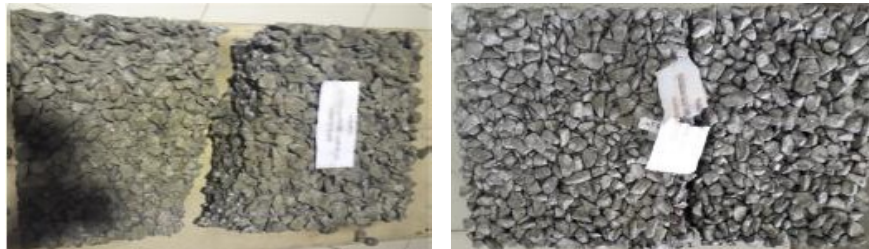
Fig. 13 - Specimen after bending test
