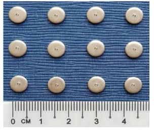
Fig. 3. Pre-drilled stainless steel discs (DEMEC pints)
