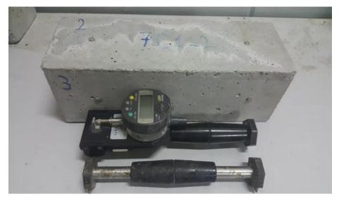
Fig. 4. The drying shrinkage measurement tool
