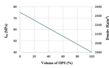
Fig 2. - Relationship between the compressive strength, substitution of OPS in NWC and dry density
