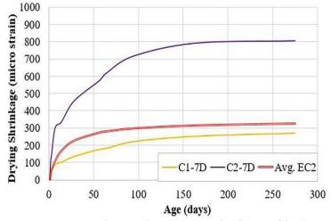
Fig. 6. Comparison and Development of the drying shrinkage for C1 and C2 mixes with EC2 model [22]
