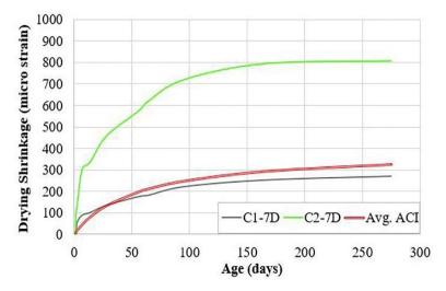
Fig. 5 - Development and comparison of the drying shrinkage for C1 and C2 mixes with ACI-209R model [21]
