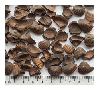
Fig 1. - Oil palm shell lightweight aggregate
