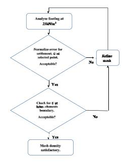
Fig. 3 - Mesh sensitivity analysis flowchart
