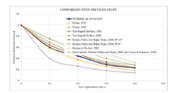
Fig. 4- Comparison of settlement reduction factors,  $\beta$  and corresponding area replacement ratios
