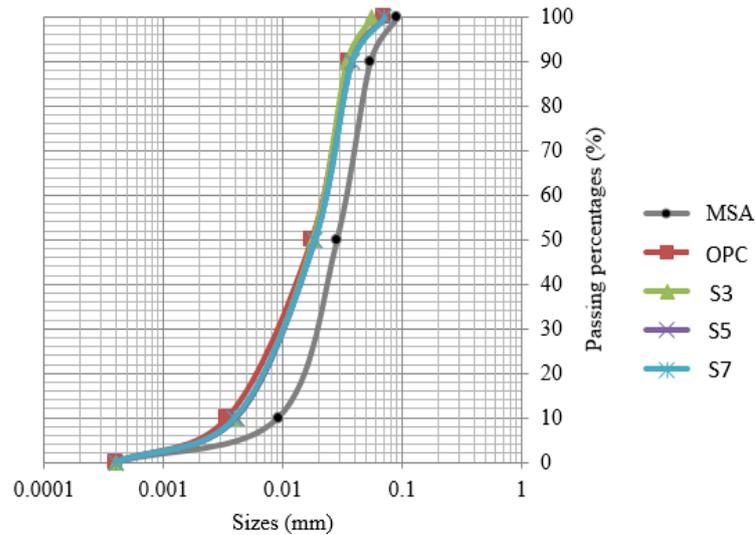
**Fig. 3 - Particle size distribution of MSA, S3, S5, S7 and OPC**
