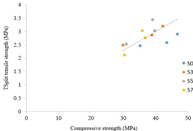
**Fig. 7 - Relationship between compressive strength and split tensile strength on 7, 28 and 60 days curing**
