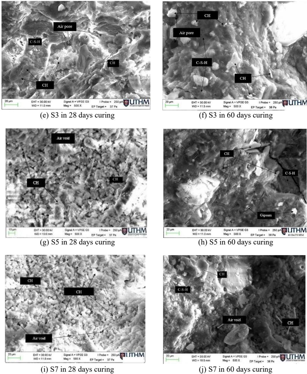
**Fig. 4 - SEM analysis of S0, S3, S5 and S7 of MSA concrete base on 28 and 60 days curing**
