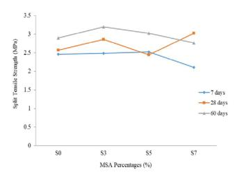
Fig. 6 - Split tensile strength of MSA concrete with different curing time
