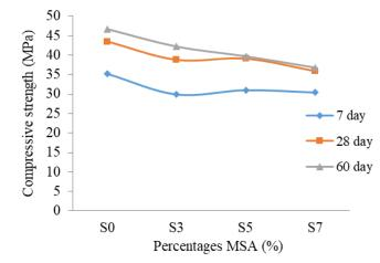
Fig. 5 - Numerical data showing the compressive strength of MSA concrete with different percentage value plotted against curing time.
