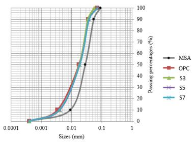
Fig. 3 - Particle size distribution of MSA, S3, S5, S7 and OPC
