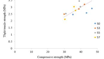
Fig. 7 - Relationship between compressive strength and split tensile strength on 7, 28 and 60 days curing
