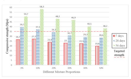
Fig. 6 - Compressive strength of different replacement percentage of CBA
