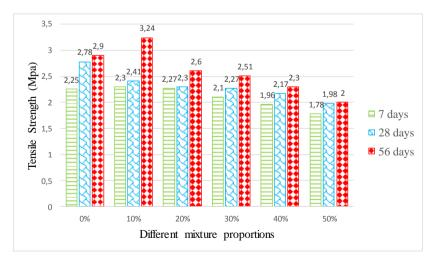
Fig. 7 - Splitting tensile strength of different replacement percentage of CBA
