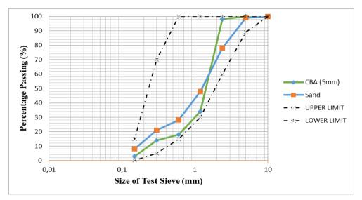
Fig. 2 - Grading analysis of CBA and sand
