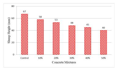
Fig. 5 - Comparison of slump height test of CBA concrete
