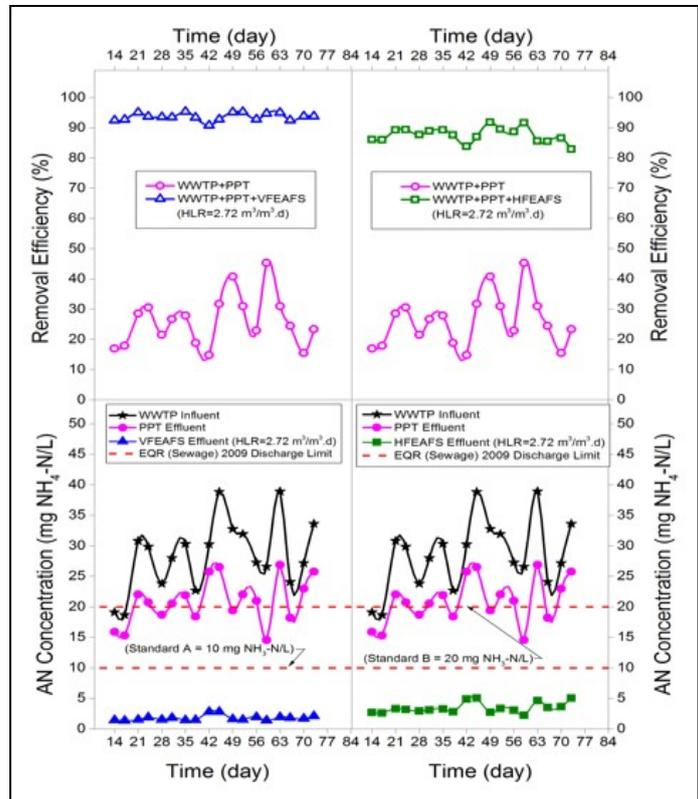
Fig. 7 - AN concentrations and removal efficiencies in the influent (WWTP) and effluents (PPT, VFEAFS filter and HFEAFS filter) sampling locations at similar HLR condition
