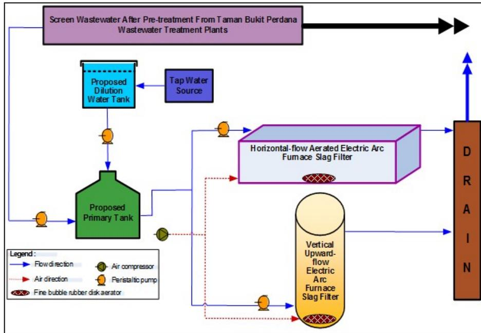
Fig. 3 - The ARFs (HFEAFS and VFEAFS) pilot-scale treatment systems layout experiment
