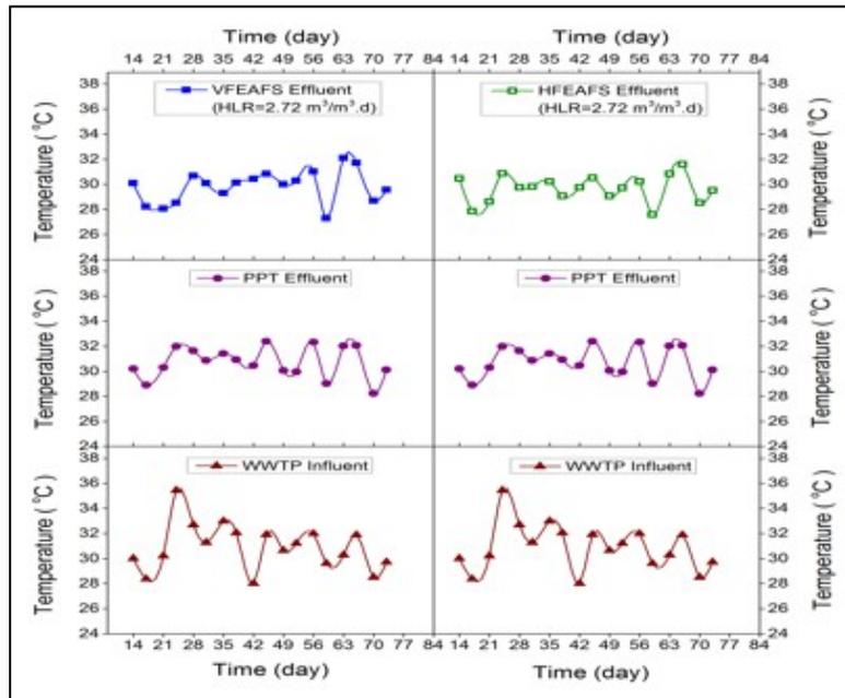
**Fig. 5 - Effluent temperature of different geometry shape of aerated EAFFS filter (vertical upward-flow and horizontal-flow) systems**
