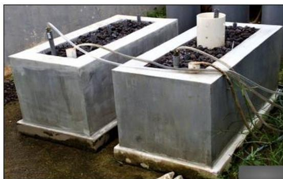
Fig. 1 - The pilot scale of horizontal-flow EAFS system at site location
