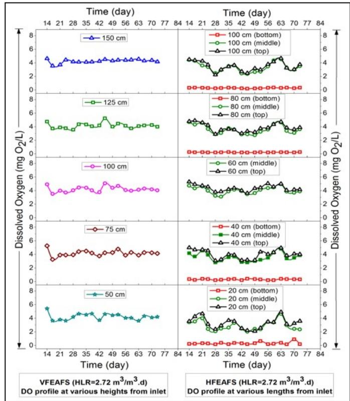
Fig. 6 - DO distribution of different geometry shape of aerated EAFS filter (vertical upward-flow and horizontal-flow systems) at various height intervals and along longitudinal direction under similar HLR operation
