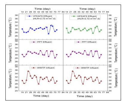
Fig. 5 - Effluent temperature of different geometry shape of aerated EAFS filter (vertical upward-flow and horizontal-flow) systems
