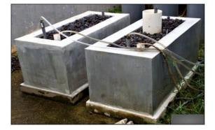
Fig. 1 - The pilot scale of horizontal-flow EAFS system at site location
