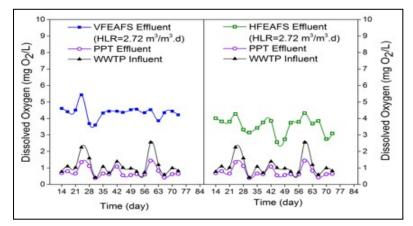
Fig. 4 - DO effluent concentrations of different geometry shape of aerated EAFS filter (vertical upward-flow and horizontal-flow) systems
