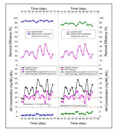
Fig. 7 - AN concentrations and removal efficiencies in the influent (WWTP) and effluents (PPT, VFEAFS filter and HFEAFS filter) sampling locations at similar HLR condition
