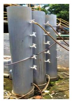
Fig. 2 - The pilot scale of vertical upward-flow EAFS system at site location
