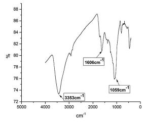
Fig. 1 - FTIR spectra of rice husk activated carbon with carbonization temperature 450°C for 20 minutes
