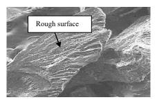
Fig. 8 - Zeolite before treatment
