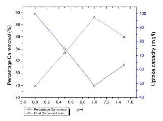
Fig. 4 - Effect of pH on the biosorption of Ca2+ onto sand, zeolite and RHAC
