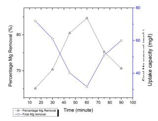
Fig. 7 - Effect of contact time on biosorption of Mg<sup>2+</sup> onto sand, zeolite and RHAC
