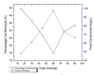
Fig. 6 - Effect of contact time on biosorption of Ca<sup>2+</sup> onto sand, zeolite and RHAC
