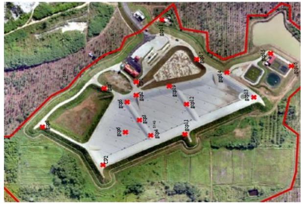
**Fig. 5 - Location of ground control point that scattered around at the landfill.**
