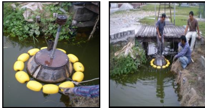
Fig. 1 - Performing the GPS buoy field test.
