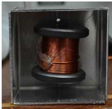
**Fig. 4 - Hand wound receiving coil with 200 turns**
