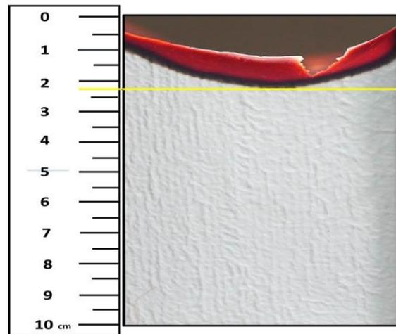
Fig. 4 - Measurement of the flame spread rate
