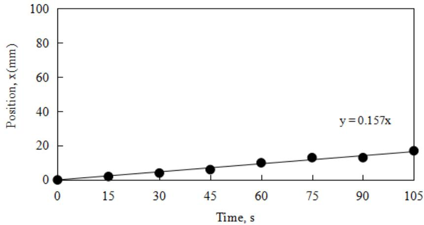
**Fig. 8 - Position of preceding point of the flame against time for 1.4mm (100% Bagasse)**
