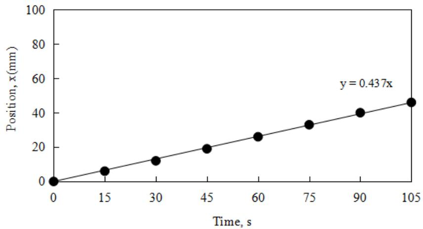
**Fig. 7 - Position of the flame against time for 2.1mm (30% Bagasse)**
