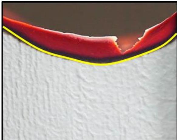
Fig. 3 - Leading edge of flame spread pattern
