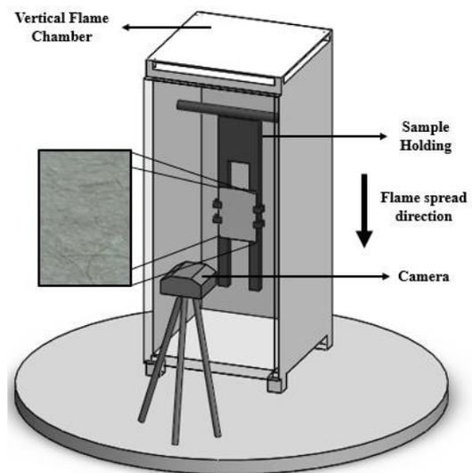
Fig. 2 - Vertical Flame Chamber
