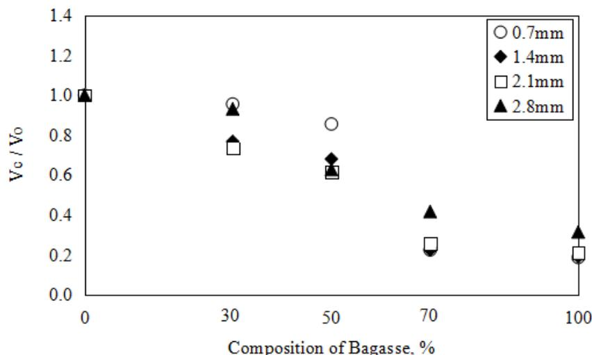
Fig. 10 -  $V_c / V_0$  against composition of bagasse
