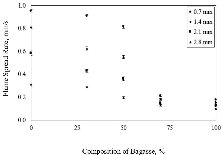
**Fig. 9 - Flame spread rate against composition of bagasse**
