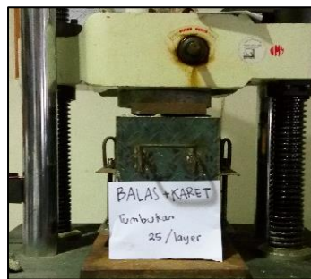
Fig. 3 - compressive test process with UTM tools.
