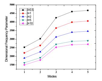
Fig 11 - Frequency parameter of first 5modes of CSCS FG square plate (Ti-6Al-4V/ZrO<sub>2</sub>) with central hole r=0.1, *b/h*=2 Tc=500K
