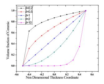
Fig 2 - Volume fraction of ceramic along the non-dimensional thickness
