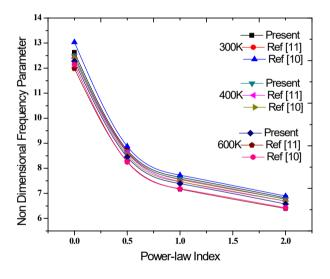
Fig 3 - Non-Dimensional Frequency of SSSS FG square Flat panel under various temperatures
