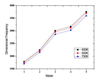
Fig 8 - Frequency parameter of first 5modes of CSCS FG square plate (Ti-6Al-4V/ZrO<sub>2</sub>) with central cutout r=0.1, b/h=5 q=1
