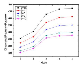
Fig 10 - Frequency parameter of first 5modes of CSCS FG square plate (Ti-6Al-4V/ZrO<sub>2</sub>) with central hole r=0.1, *b/h*=2 Tc=400K
