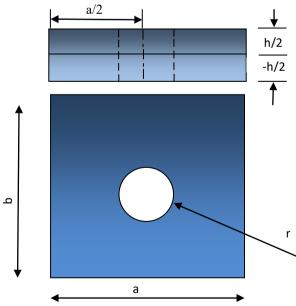
Fig. 1 - Elevation and plan of functionally graded plate with central hole
