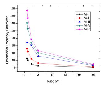
Fig 5 - Vibration responses of first 5modes of CFFF FG square plate (Ti-6Al-4V/ZrO<sub>2</sub>) with central hole r=0.1, q=2 T<sub>c</sub>=500K
