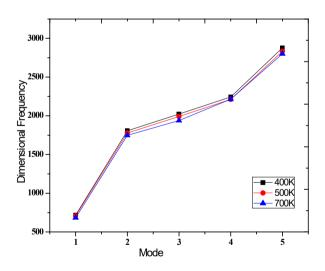
Fig 7 - Frequency parameter of first 5modes of simply supported FG square plate (Ti-6Al-4V/ZrO<sub>2</sub>) with central cutout *r*=0.1, *b/h*=5 *q*=1
