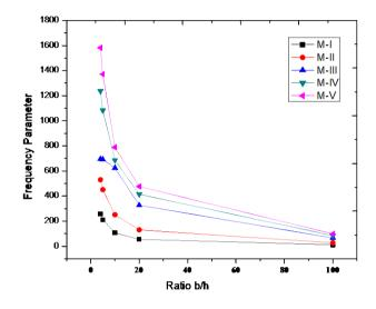
Fig 4 - Frequency parameter of first 5modes of CFFF FG square plate (Ti-6Al-4V/ZrO<sub>2</sub>) with central hole r=0.1, q=2 Tc=400K
