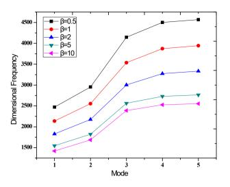
Fig 12 - Frequency parameter of first 5modes of CSCS FG square plate (Ti-6Al-4V/ZrO<sub>2</sub>) with central hole r=0.1, *b/h*=2 T<sub>c</sub>=700K
