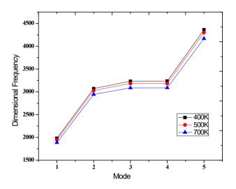
Fig 9 - Frequency parameter of first 5modes of CCSS FG square plate (Ti-6Al-4V/ZrO<sub>2</sub>) with central cutout r=0.1, b/h=5 q=1
