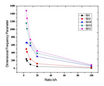
Fig 6 - Frequency parameter of first 5modes of CFFF FG square plate (Ti-6Al-4V/ZrO<sub>2</sub>) with central hole r=0.1, q=2 Tc=700K
