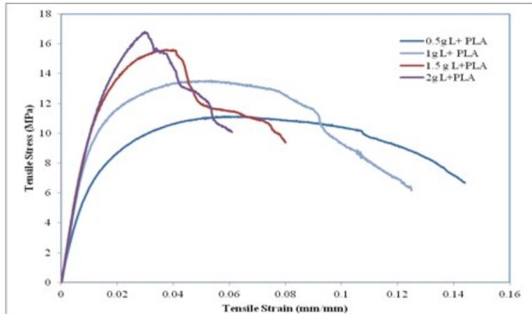
Figure 1 - Tensile strength of the composite films with varying natural fiber powder loading
