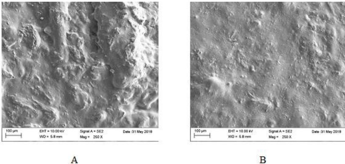
Figure 2 - a. SEM image of 0.5 gms luffa cylindrical reinforced composite b. SEM image of 2 gms luffa cylindrical reinforced composite.
