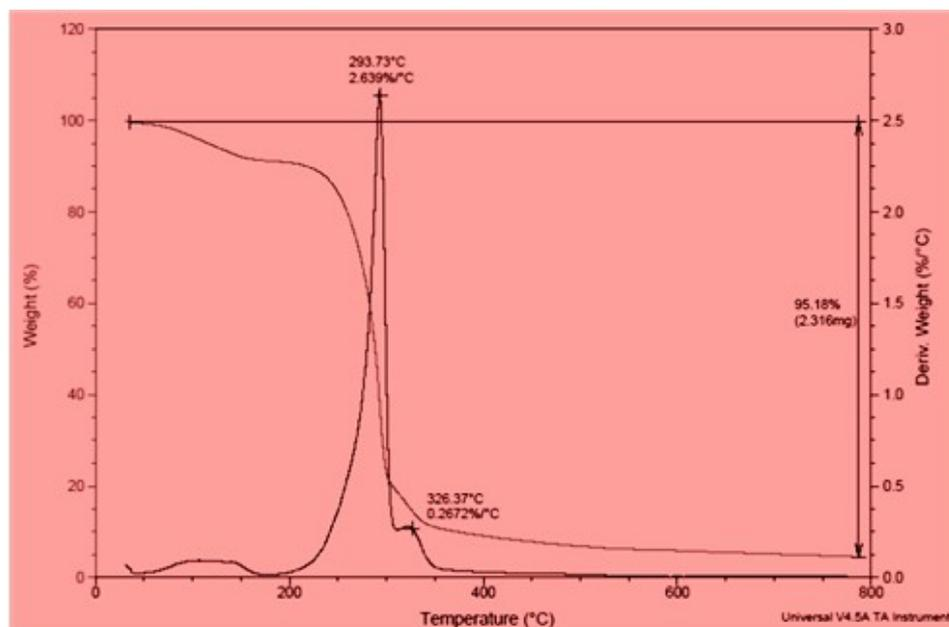
Figure 6 - TGA graph of 1 gram Luffa cylindrical reinforced composite film
