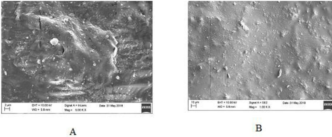
Figure 3 - a. SEM image of 0.5 gm luffa cylindrical reinforced composite at  $2\ \mu\text{m}$  b. SEM image of 2 gm luffa cylindrical reinforced composite at  $10\ \mu\text{m}$
