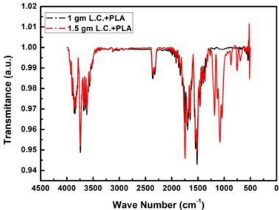
Figure 4 - FTIR graphs of both 1 gm and 1.5 gm luffa cylindrica reinforced composite films
