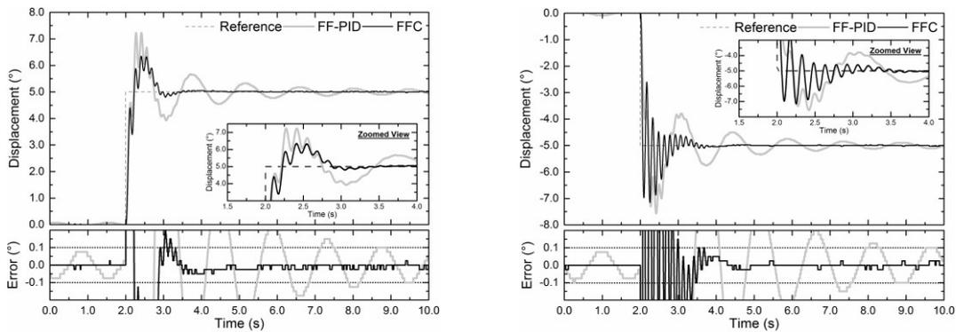
**Fig. 5 - Comparative step response of FFC and FF-PID controller at (a)  $5.0^\circ$ ; (b)  $-5.0^\circ$**
