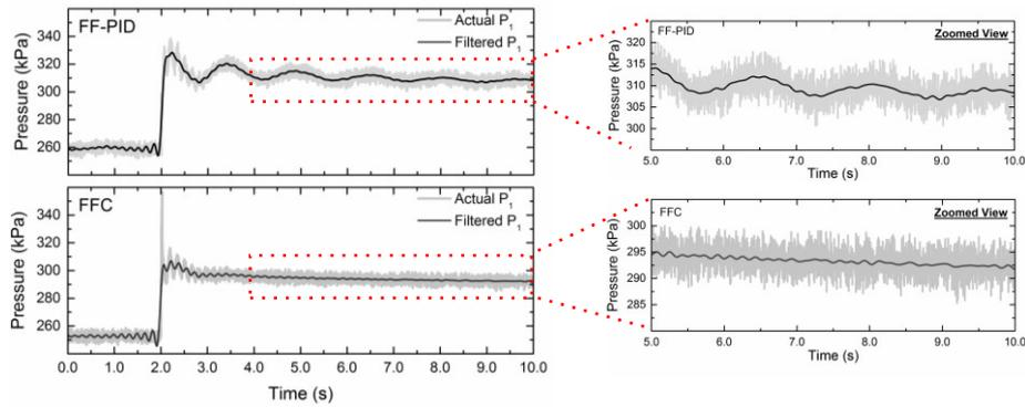
Fig. 7 - Comparative pressure response of FFC and FF-PID controller at 10.0°
