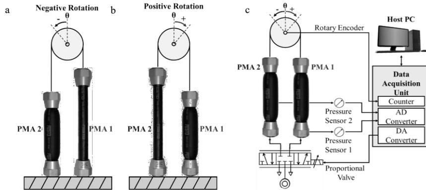
**Fig. 3 - (a) Operation of system in negative direction; (b) Operation of system in positive direction; (c) Experimental setup for antagonistic based PMA system**
