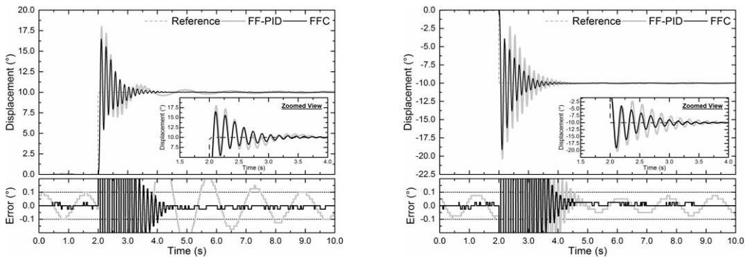
**Fig. 6 - Comparative step response of FFC and FF-PID controller at (a)  $10.0^\circ$ ; (b)  $-10.0^\circ$**
