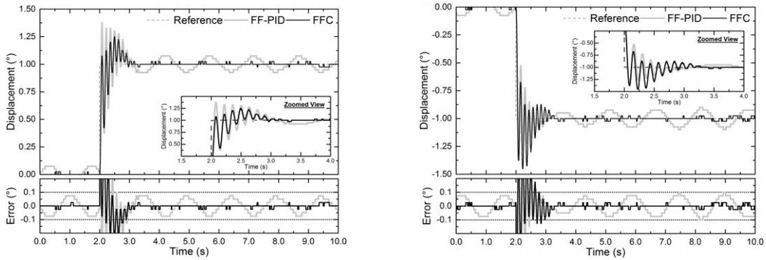
**Fig. 4 - Comparative step response of FFC and FF-PID controller at (a)  $1.0^\circ$ ; (b)  $-1.0^\circ$**
