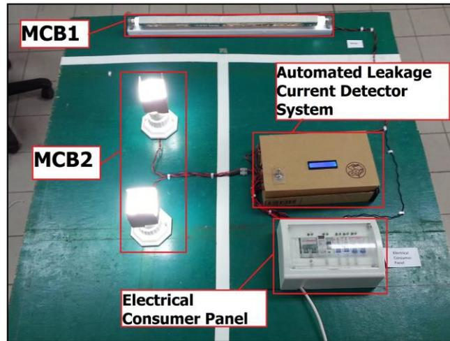
Fig. 5 - Overview of the prototype
