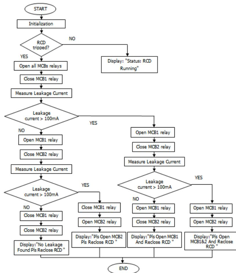
Fig. 6 - Software programming flow
