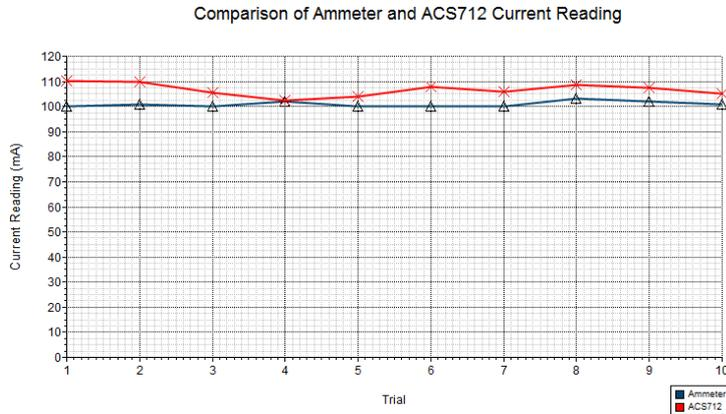
**Fig. 3 - Comparison of Ammeter and ACS712 Current Reading**
