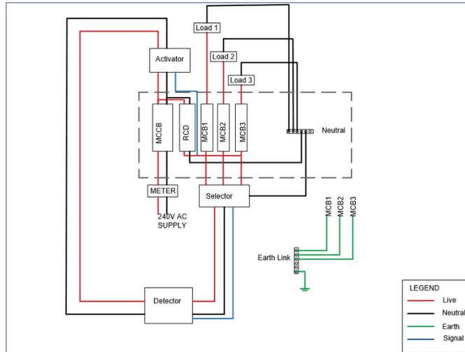
**Fig. 2 - Pre-designed block diagram**
