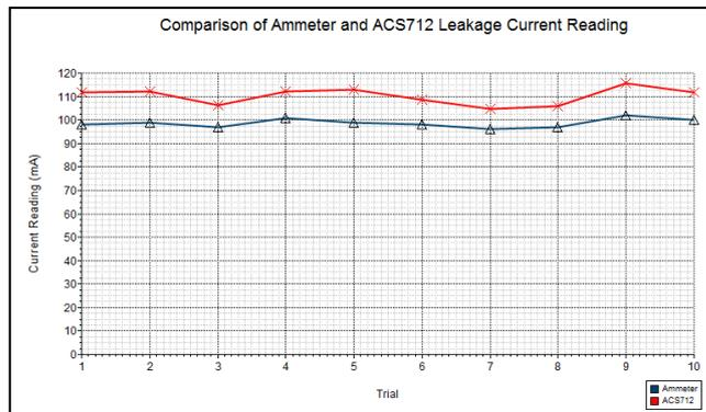
**Fig. 4 - Comparison of Ammeter and ACS712 Leakage Current Reading**
