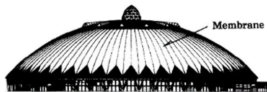
Fig.1: Example of framed membrane structures [6].
