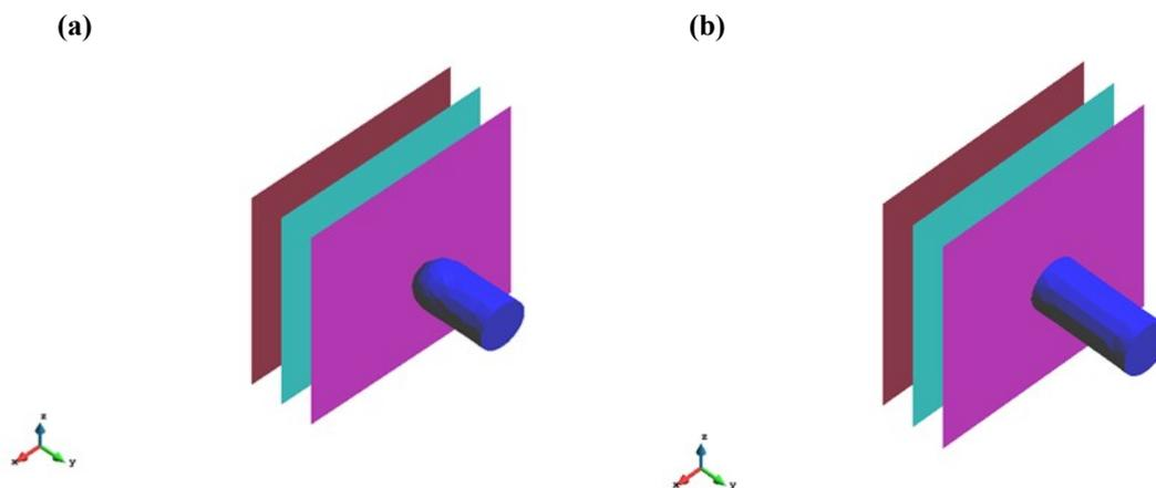
**Fig. 1 - Finite element model of projectile and multilayer target plate**
