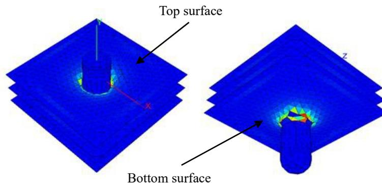
**Fig. 5 - Failure mode of model impacted by a hemispherical bullet at a velocity of 22m/s**
