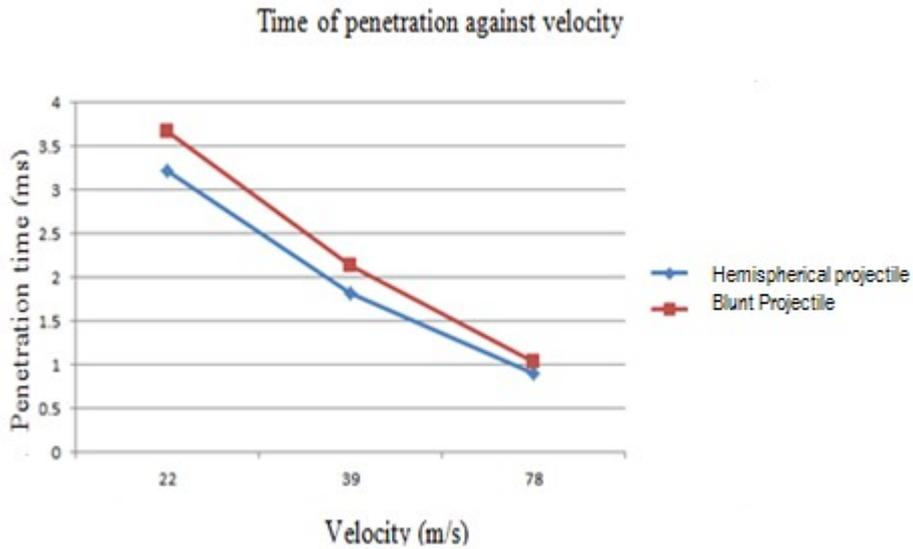
**Fig. 6 - Graph of time taken for bullet to complete penetration at a different velocity**
