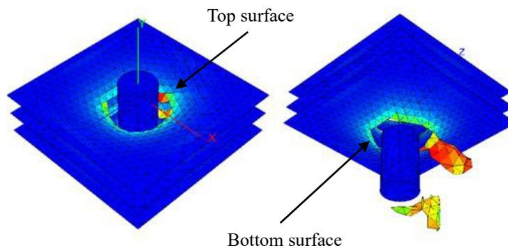
**Fig. 4 - Failure mode of model impacted by blunt bullet at velocity of 22m/s**
