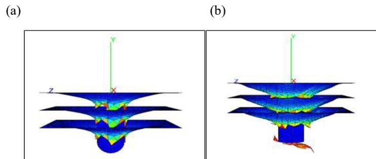
**Fig. 9 - Failure mode geometry of target plate impacted at velocity of 78m/s
