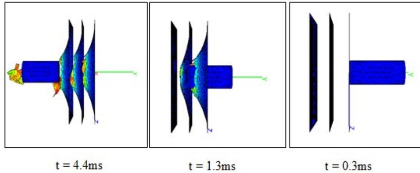
**Fig. 8 - Plug formation of blunt nose projectile impacted on the multilayer target plate**
