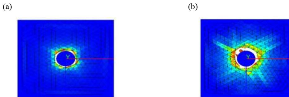
**Fig. 7 - Top view images of post penetration of projectile (a) Hemispherical nose shape (b) Blunt nose shape**
