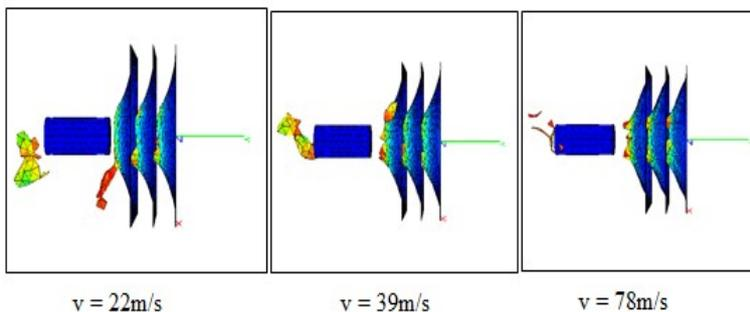
**Fig. 3 - Penetration at different velocity impact (a) Hemispherical projectile impact (b) Blunt projectile impact**
