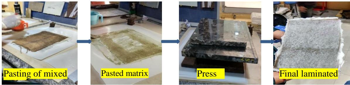
**Fig. 2 - Fabrication of composite laminate**
