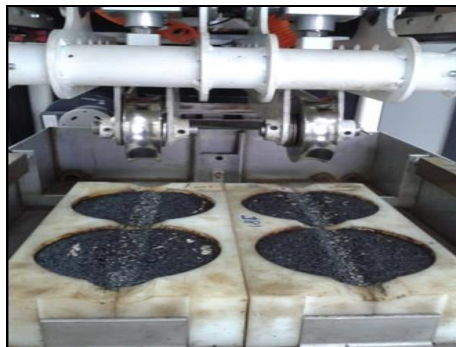
Fig. 4 - Specimen after the APA test.
