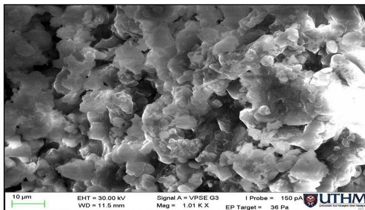
Fig. 12 - SEM image sludge leachate at dose 3g/L of PAC.
