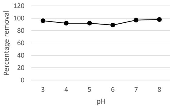
**Fig. 7 - Percentage removal of suspended solid of varied pH at dose PAC 4g/L.**
