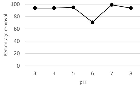
**Fig. 4 Percentage removal of suspended solid of varied pH at dose PAC 3g/L.**
