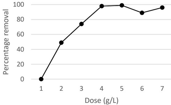
**Fig. 1 - Removal of suspended solid of varied dose of PAC at pH 7.**
