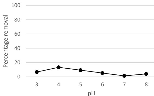
**Fig. 11 - Removal of suspended solid of varied pH at dose 1.0g/L of tapioca flour.**
