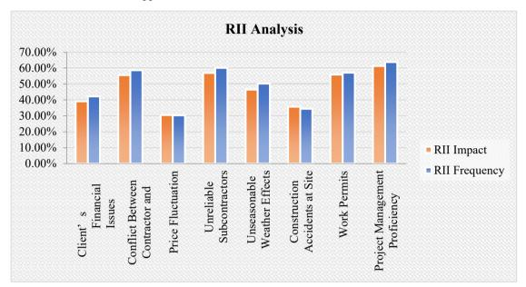
Figure 2 - An illustration of the Relative Importance Index for every external factor of delay
