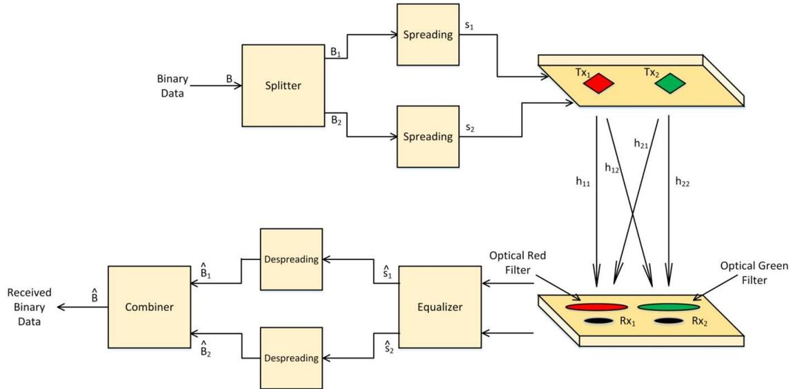
**Fig. 1 – System modeling of proposed CSK-CDMA based indoor VLC system**
