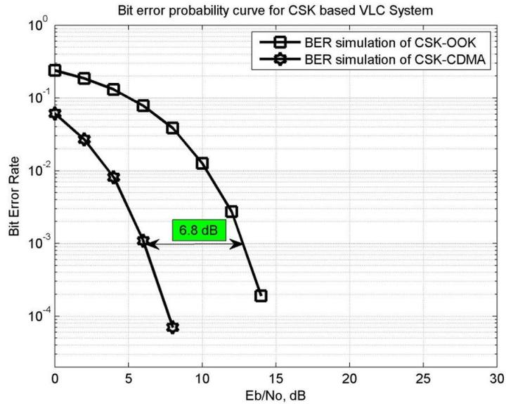
**Fig. 2 – Performance comparison of proposed and traditional CSK based VLC system**
