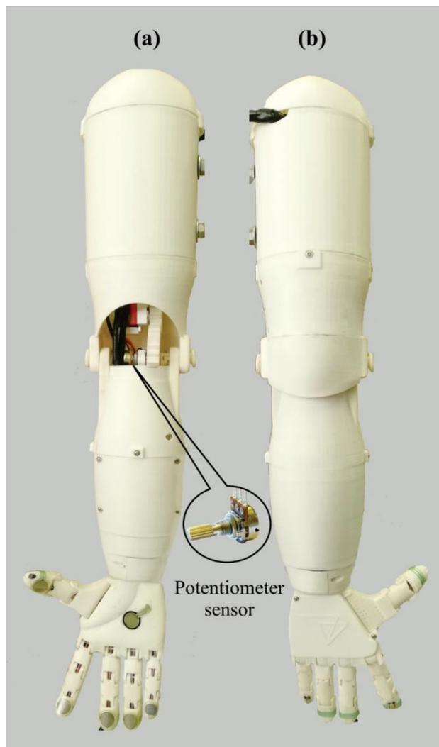
Fig. 2 - Fabrication of the tactile prosthetic arm: a) front view, and b) rear view
