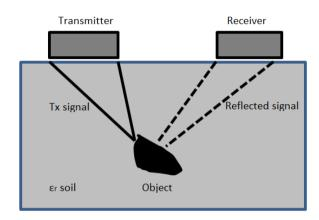
Fig. 1 - Bi-Static GPR System
