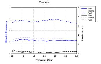
Fig. 11 - Dielectric properties of concrete
