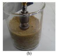
Fig. 5 - Measured samples, (a) Dried sand (b) Wet sand
