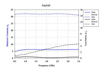
Fig. 6 - Dielectric properties for asphalt
