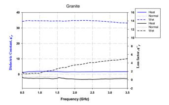
**Fig. 8 - Dielectric properties of granite**
