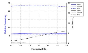
Fig. 10 - Dielectric properties of fine sand
