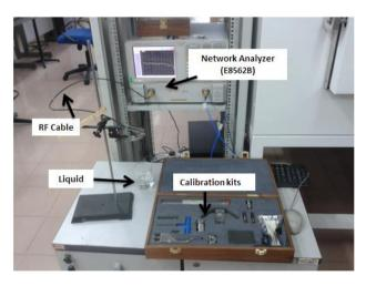
Fig. 4 - Dielectric Coaxial Probe and Calibration Kits
