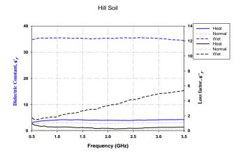
Fig. 9 - Dielectric properties of hill soil.
