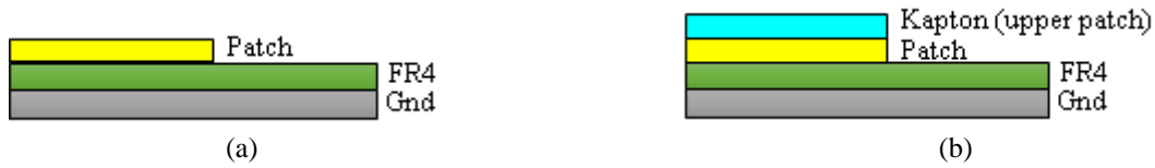
Fig. 2 - Microstrip patch antenna design (side view), (a) Design A – without kapton and (b) Design B to J with Kapton
