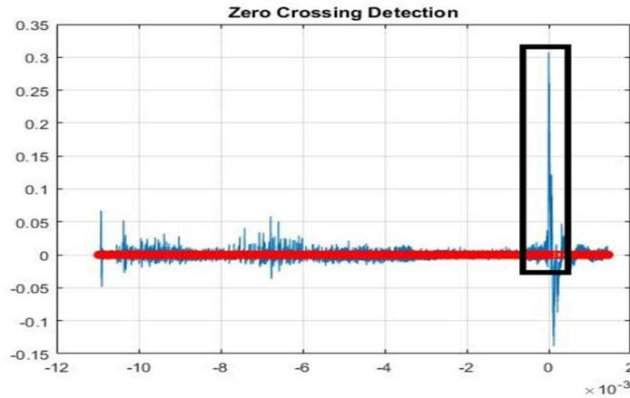
**Fig. 5 - The figure shows the whole event starting from the preliminary breakdown pulses until the first return stroke. The rectangular box marker highlighted in black is the first return stroke signal.**
