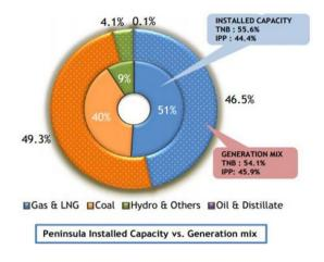
Fig.1 - Peninsula Malaysia installed capacity vs. generation mix
