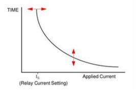
Fig. 4 - Standard IDMT characteristic
