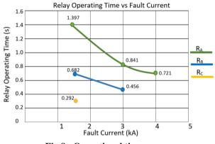
Fig.8 - Operational time curve
