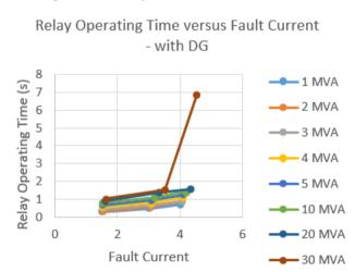
Fig. 11 Relay operating time vs fault current
