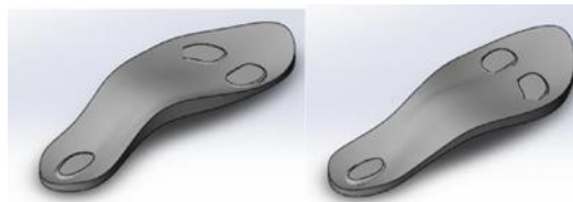
Fig. 10 - 3D model of orthotics insole.
