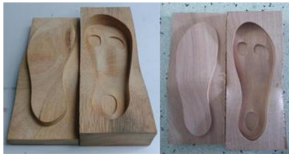
Fig. 13 - Wood mould of orthotics insole (male and female)
