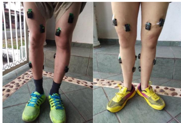
Fig. 19 - Sensor placement in lower limb muscles (male and female).
