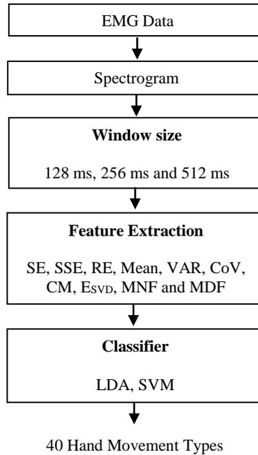
**Fig. 1 - Flow diagram of the pattern recognition architecture.**
