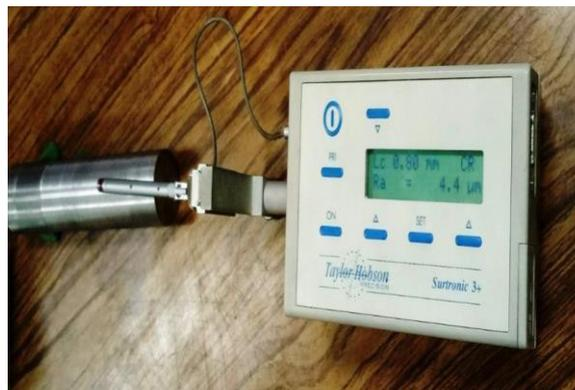
Fig. 4 - Surface Roughness Measurement instrument
