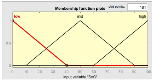
**Fig. 5 - The membership functions of the input, SoC**
