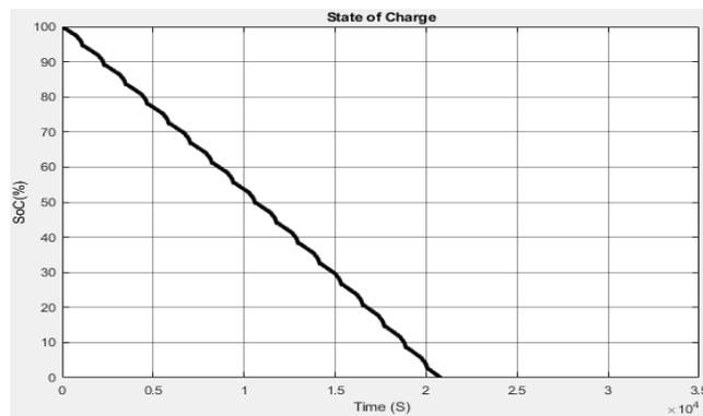
**Fig. 9 - Soc of the Basic Model with HVAC Full-Unmanaged Load (NEDC)**
