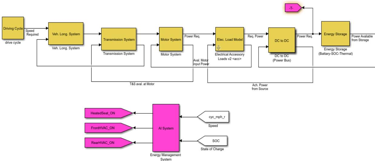
Fig. 3 - BEV Model Simulation with Fuzzy Logic Controller
