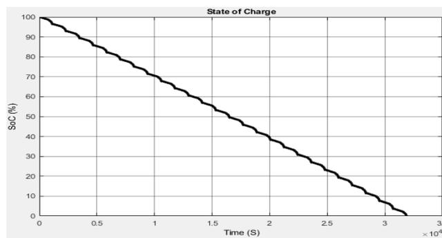
Fig. 7 - SoC of the Basic Model with No HVAC Load (NEDC)
