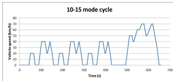
**Fig. 2 - Japan 10-15 Driving Cycle [9]**
