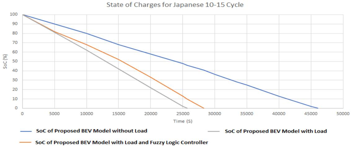
Fig. 14 - SoC Comparison Diagram Between the Three Scenarios (Japan 10-15)
