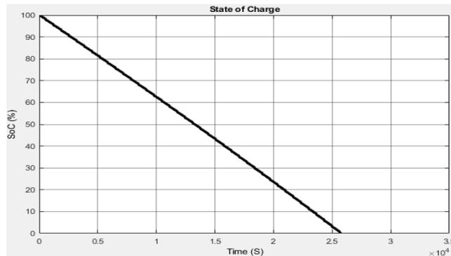
**Fig. 10 - SoC of the Basic Model with HVAC Full-Unmanaged Load (Japan 10-15)**
