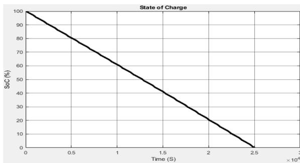
**Fig. 11 - SoC of the Fuzzy Logic Integrated Model with HVAC Controlled Load (NEDC)**
