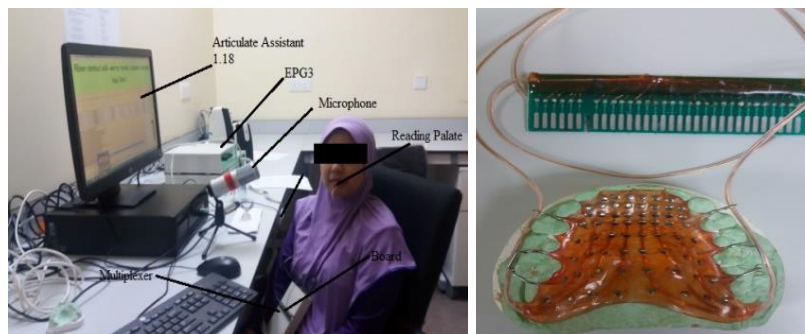
Fig. 1 - EPG system and the Reading palate with 62 silver electrodes
