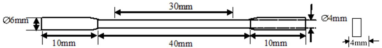
Fig. 1 - Specification for tensile coupons
