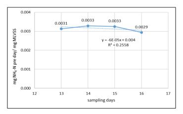
Fig. 6 - mg NH4-N per day/ mg MLVSS vs sampling days
