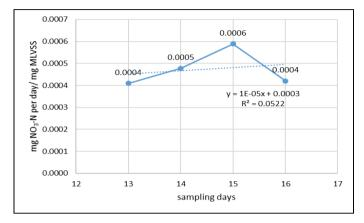
Fig. 7 - mg NO<sub>3</sub>-N per day / mg MLVSS vs sampling days
