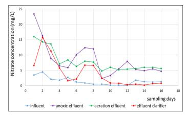
Fig. 3 - Characteristic for nitrate concentration
