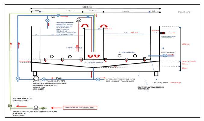
Fig. 1 - Schematic diagram of the i-SGS pilot plant
