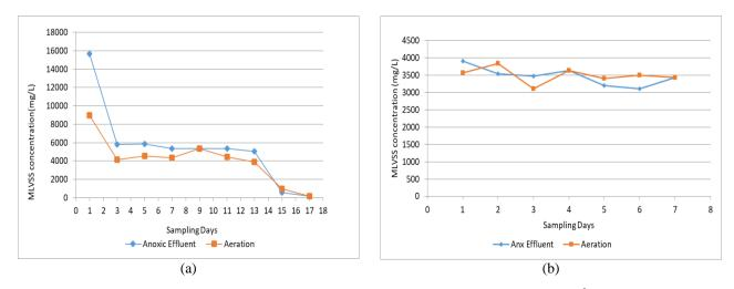
Fig. 4 - MLVSS concentration (mg/L) vs sampling days (a) 1<sup>st</sup> run, (b) 2<sup>nd</sup> run
