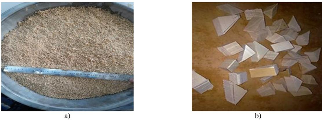
**Fig. 1 - Wood wast: a) sawdust waste, and b) wood waste aggregate.**
