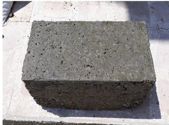
**Fig. 4 - Concrete block unit specimen.**
