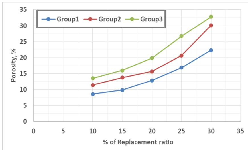
Fig. 8 - Relationship between porosity and replacement ratio.
