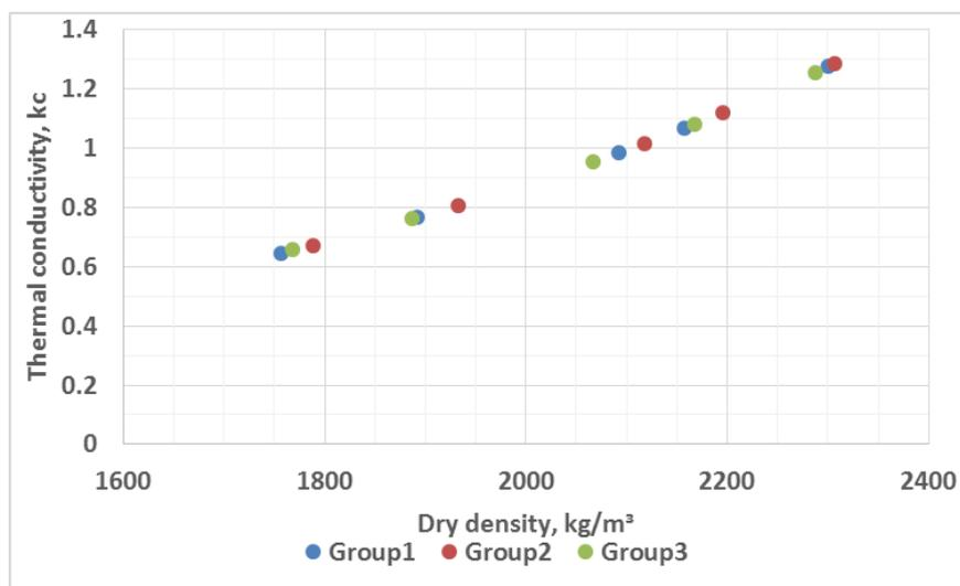
Fig. 10 - Coefficient of thermal conductivity,  $k_c$  versus dry density.
