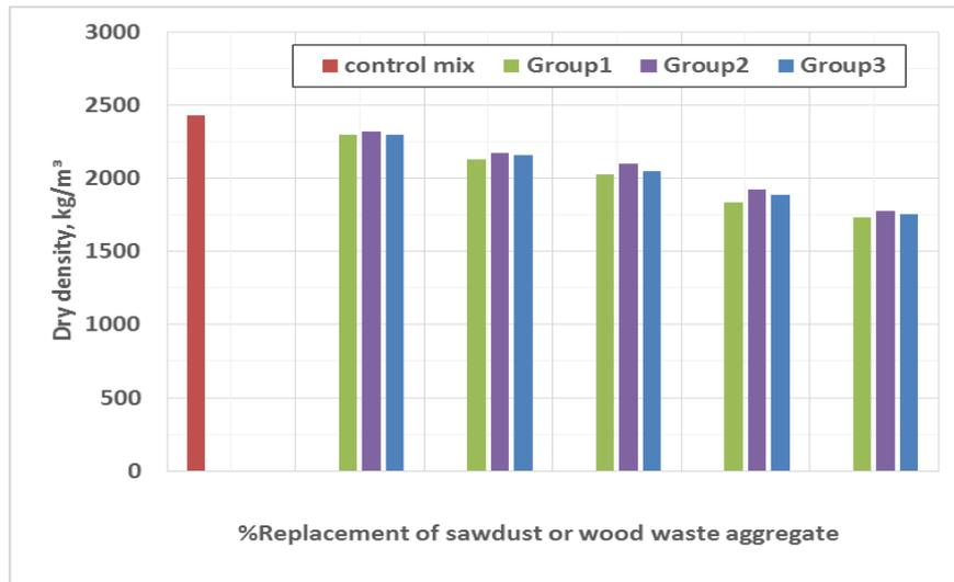
Fig. 7 - Reduction of dry density versus % sawdust and wood waste aggregate.
