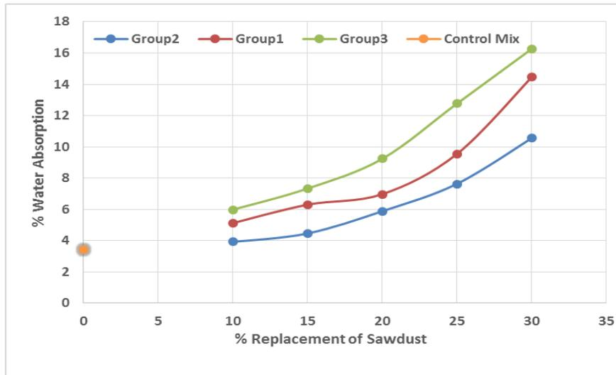
Fig. 6 - Relationship between water absorption and % sawdust and wood waste aggregate.
