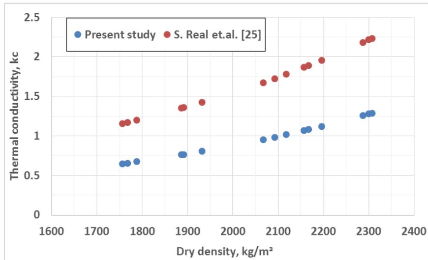
Fig. 11 - Coefficient of thermal conductivity,  $k_c$  in present study as compared to Real et al. [25].
