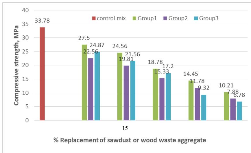
Fig. 5 - Compressive strength versus % sawdust and wood waste aggregate in mixes.
