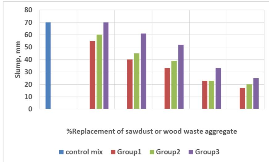
Fig. 9 - Slump versus % sawdust waste and wood waste aggregate.
