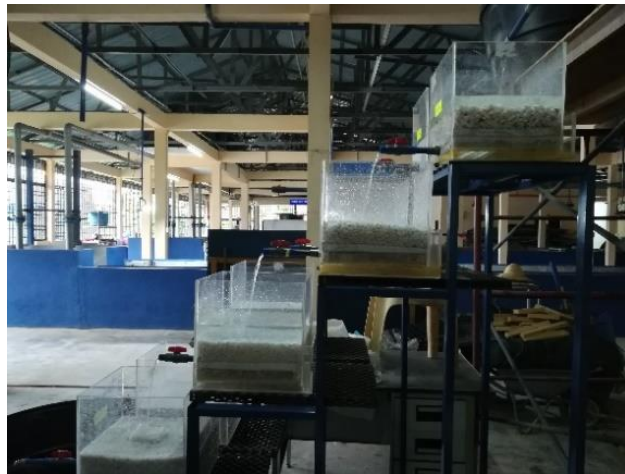
Fig. 1 - Side view of marble column filter which arranged in increasing grain size from bottom to top column
