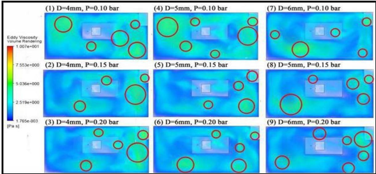
Fig. 8 - Eddy viscosity diagram of P=0.10 bar, P= 0.15 bar and P=0.20 bar for D=4mm, D=5mm and D=6mm
