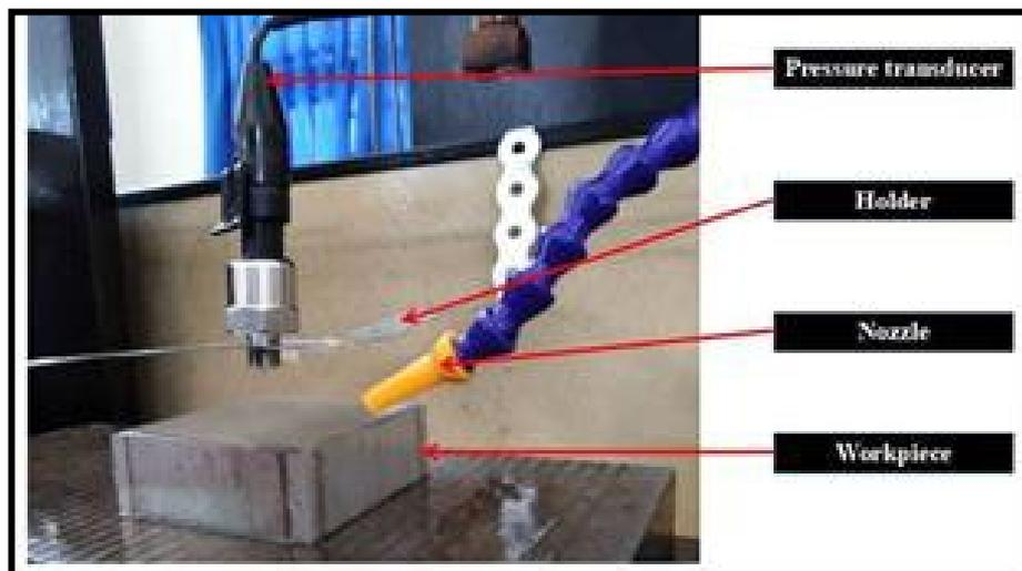
Fig. 1 - Setup of pressure transducers
