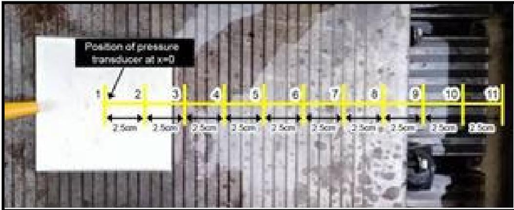
Fig. 2 - The eleven positions of pressure transducer
