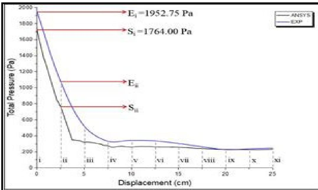
Fig. 9 - Total pressure by using case 5 for validation result by comparing the experimental data and FLUENT result
