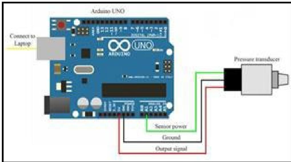
Fig. 3 - Wiring schematic diagram for installation of pressure transducer and Arduino
