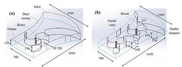
Fig. 1 - Savonius wind turbine model for (a) reference model; b) modified model. Dimensions are in mm
