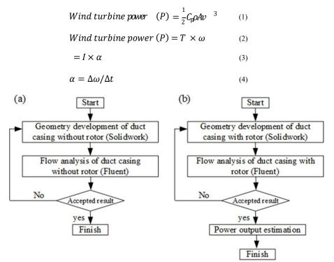
Fig. 2 - Analysis flowchart for (a) Duct casing without rotor; (b) Duct casing with rotor
