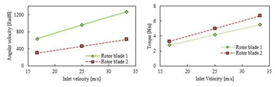
Fig. 6 - The performance of rotor blade 1 and 2 for (a) Angular velocity; (b) Torque as a function of inlet velocity
