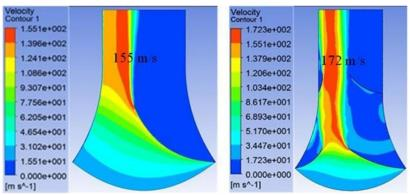
Fig. 3 - Velocity contour of duct casing without rotor for (a) reference model; (b) modified model
