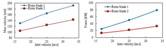
Fig. 5 - The performance of rotor blade 1 and 2 for (a) Maximum velocity; (b) power output as a function of inlet velocity
