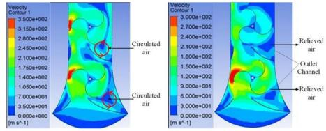
Fig. 4 - Velocity contour of modified model (duct casing with rotor) (a) without; (b) with additional outlet channel
